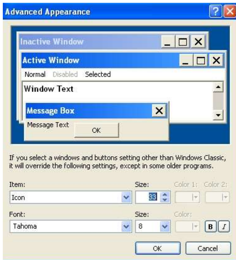
Figure 4: Changing the size of an icon (Item) and the size of the icon text (Font).
